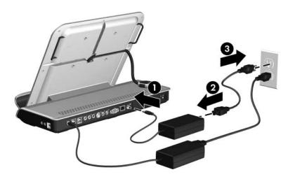
Connecting the Hard Drive AC Adapter
